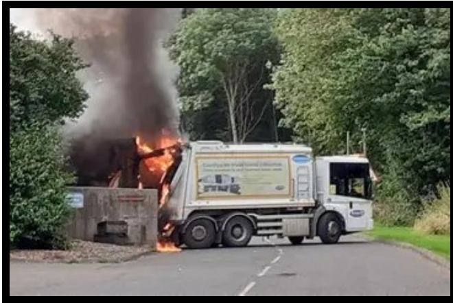
Refuse collection vehicle ablaze — discarded batteries, vapes and e-scooters in the waste stream are a fast-growing cause of RCV fires across the UK.
