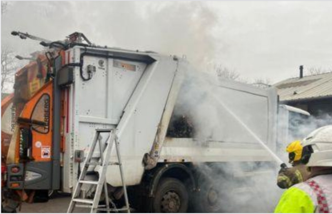
Firefighters tackling a refuse lorry fire caused by lithium-ion battery ignition.
